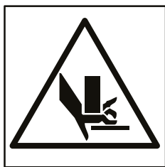
Crush hazard - moving parts
