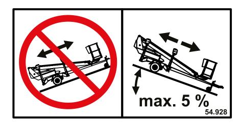
Do not drive downhill with the driving device, if the inclination of the surface is more than 5 per cent, (corresponding to a descent of 0.5 m over a distance of 10 m). If the gradient of the surface is greater than this, you may lose control of the device.
