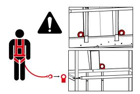
Ensure that the gates are properly closed before starting the operation. If the work platform is equipped with ladder, these must be locked in the upper position.
