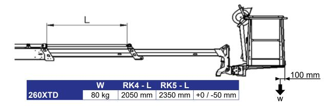
The red warning light for overloading will illuminate as soon as the **RK4** has stopped the movement. While at the outreach limit, the red warning light and the green signal light will flash in turns. In this situation, the lift can be operated in the direction, in which it remains inside the permitted outreach area.
