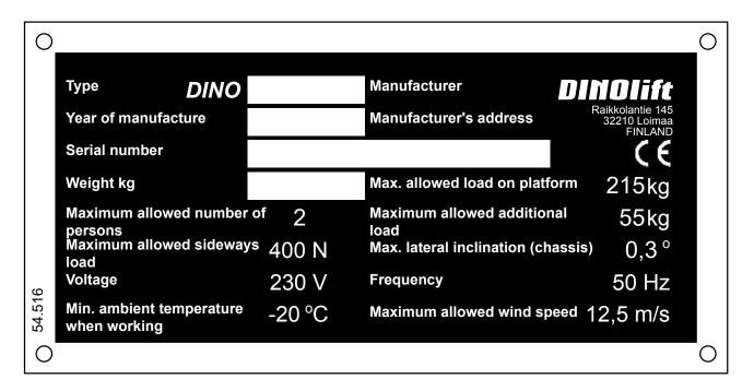
The nameplate of the lift is located on the right-hand side of the tow-bar, as shown in the picture.
