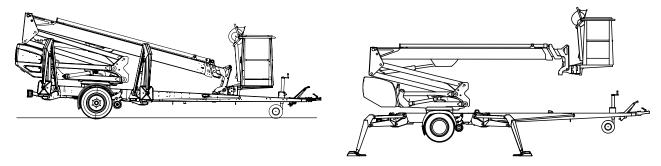
The primary power source of the lift is the electric motor. The outriggers and the boom system are hydraulically powered.
