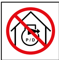
Running the engine indoors prohibited
