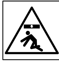
Crush hazard - falling objects
