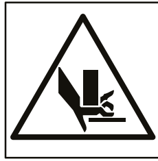
Crush hazard - moving parts
