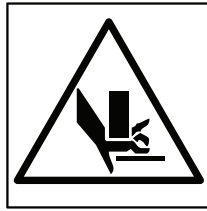
Risk of getting crushed - moving parts
