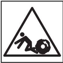
Risk of getting crushed - moving parts
