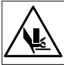
Risk of getting crushed - moving parts
