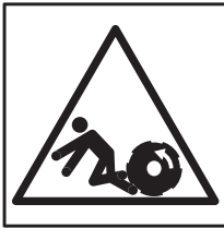
Risk of getting crushed - moving parts
