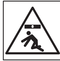
Risk of getting crushed - falling objects
